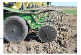
The **closing wheels** close the seed trench behind the seed. The chains level the dirt behind the closing wheels.
