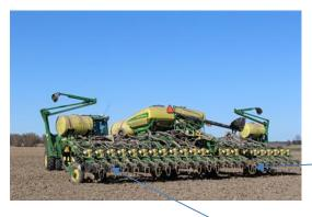
A **planter** is a farm implement, usually towed behind a tractor, that sows (plants) seeds in rows. It is connected to the tractor with a drawbar or a three-point hitch. The picture above has a single **seed box** that is filled, and then air pressure blows the seed to the seed boxes. A **seed meter** drops the seed into the seed tube. The **seed tube** then drops the seed into the seed trench.
