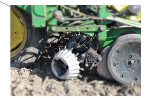
A **no-till coulter** breaks up the ground ahead of the **disc opener blades** and **seed tube**, so the seed can reach a well-prepared seed bed. The **disc openers** create the slot for the seed tube to drop the seed in.
