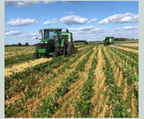
A combine (right) harvests the wheat while a baler (left) bales the stalks for straw. The soybeans, which were interseeded into the standing wheat remain.
